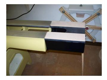
Tailstock assembly slid onto and locked to removal unit. Note: Prop stick is only for photograph purposes.
