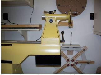
Hard maple and MDF removal unit in position. Note the u-shaped channel which prevents the tailstock assembly from sliding off the removal unit.
